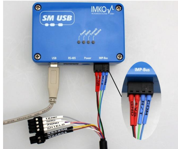
Wiring with end splices via IMP-Bus
