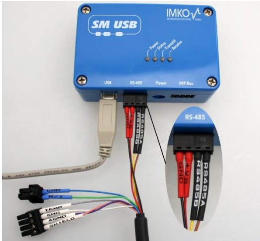
Wiring with end splices via RS485
