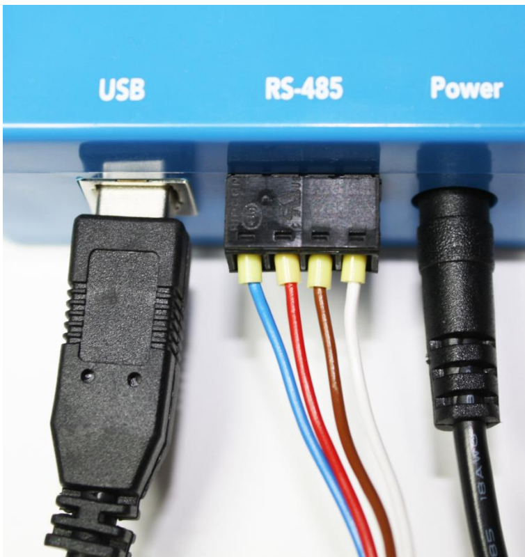
Detailed wiring for SONO-Probes connection via RS485
