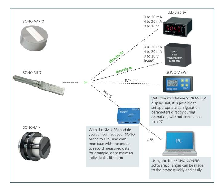
Predictive sensor networking through intelligent device communication ensures smooth processes in the application. The IMP bus does not transmit its data packets as voltage pulses, but as current pulses. Thus, the process works even with long cable lengths on existing and already laid lines. A shielded cable is not required and even spurs in wide-ranging network topologies are not a problem.
