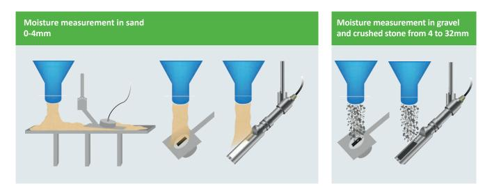
As well as using the right measurement technology, the efficient functioning of a moisture sensor relies on faultless mechanical integration.
