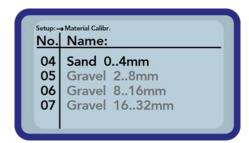
The list can be scrolled and the desired calibration be selected by actuating the buttons "Up" and "Down" . The "!" in front of a calibration indicates the currently active one. You can set the selected calibration to become the active one by actuating the button "Measurement" . After a short moment, the symbol will appear in the upper right hand display corner to indicate that the selection has been activated. In addition, the "!" will be placed in front of the now active calibration.
