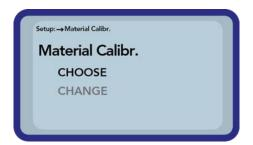
After the selection of the menu item "Material Calibration", you have to choose between "CHOOSE", to save one out of fifteen calibration as default calibration, or "CHANGE", to setup an individual new calibration in one of the fifteen calibration storages.
