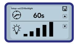
The selection of the background illumination, respectively the time until the automatic shut-down of it is selected via the button "Up" by actuating it several times. Using the button "Down" , is used to adjust the intensity of the illumination, respectively turn the same completely off. Activate and store your settings by actuating the button "Measurement" . After activation, the symbol will appear in the upper right-hand corner of the display.
