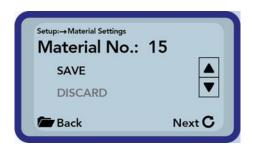
Finally, you can store the calibration into the choosen calibration storage inside the probe. Choose "SAVE" and confirm by pressing the button "Measurement" . If you choose "DISCARD" everything is left untouched.
