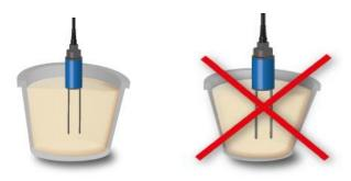
The filling depth of the bucket must exceed the rod length by minimum 5cm
