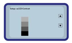
Change the contrast by actuating the button "Up" △, respectively "Down" ☑. Set the contrast that you can realize the whole grayscale on the diagram. Activate and store your settings by actuating the button "Measurement" ☑. After activation, the symbol ☐ will appear in the upper right hand corner of the display.
