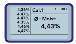
8 In total six averaged measurements are available now. The representative value for the probe is the average value out of these six measurements.
