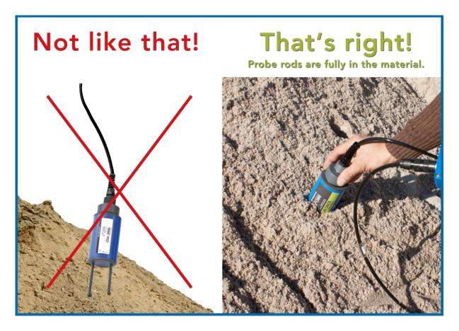
To obtain a representative moisture value of the material, select the operating mode "Average Value" and take measurements at different locations.
