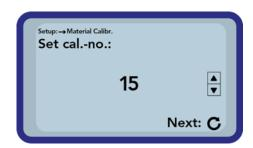
First you have to set the calibration curve to be changed (01 - 15) by pressing the buttons "Up" and "Down" . Apply your setting by actuating the button "Measurement"
