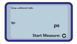
To start the measurement of the material press the button "Measurement" . To improve the accuracy, four measurments will be taken. The individual values are averaged. The duration of a measurement takes around 20 seconds. After each measurement the signal runtime will be displayed for a short period.
