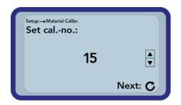
First you have to set the calibration curve to be changed (01-15) by pressing the buttons "Up"  $\triangle$  and "Down"  $\square$ . Apply your setting by actuating the button "Measurement"  $\square$
