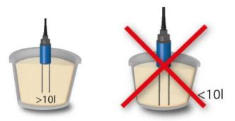
• The bucket should be as far as possible cylindrical, to prevent compaction of the material.
