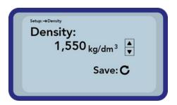
Adjust the density of your material by actuating the buttons "Up" and "Down" . Confirm your setting by pressing the button "Measurement" . You will get back to the measurement screen. Leave the setting without changing the density by pressing the button "Settings".
