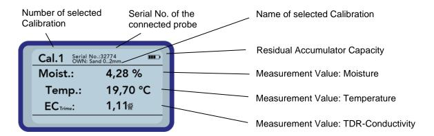
In order to initiate a measurement, shortly press the button "Measurement" . The measurement will commence and a turning . -symbol will appear instead of the accumulator-symbol in the upper right hand corner. During this period, no other actions can be performed. The measurement requires approximately 4 to 5 seconds.
