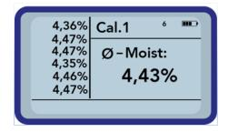
Within the operating mode "Average Value", the HD2 will deliver a representative measurement result for the volume of the material.
