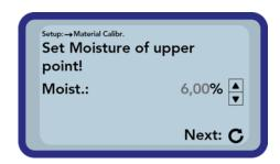
Next set the moisture of the higher moisture point by pressing the buttons "Up" → and "Down" ✓. Apply your setting by actuating the button "Measurement " ⊙.
