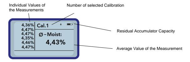
In order to initiate a measurement, shortly press the button "Measurement" . The measurement will commence and a turning -symbol will appear instead of the accumulator-symbol in the upper right-hand corner. During this period, no other actions can be performed. The measurement requires approximately 4 to 5 seconds.
