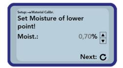
Next set the moisture of the lower moisture point by pressing the buttons "Up" ▲ and "Down" ▼.
