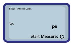
To start the measurement of the material press the button "Measurement" . To improve the accuracy, four measurements will be taken.
