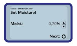
Next set the moisture of the material by pressing the buttons "Up" and "Down" . Apply your setting by actuating the button "Measurement" .
