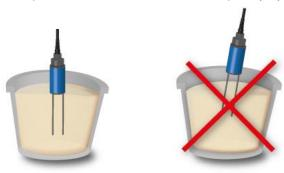
The bucket must have a volume of 10 liters or more. Never use a metal bucket, the metal is disturbing the measurement field of the probe.
