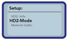
By actuating the buttons "Up"  $\triangle$  and "Down"  $\bigvee$ , the entry intended for processing can be marked and subsequently be selected with the button "Measurement"  $\bigcirc$ . You can exit the current menu item and also the menu "Settings", with the button "Settings"  $\bigcirc$ .
