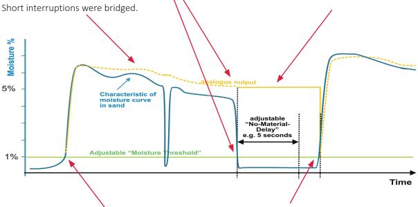
Start of first batch process. The SONO-probe recognizes that the adjustable moisture threshold of e.g. 1% has been exceeded and the probe starts automatically with the continuous accumulation of measurement values (yellow curve).
