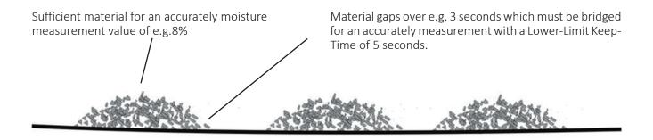
The following parameter setting in mode CA fits a high pass filtering for bridging material gaps.
