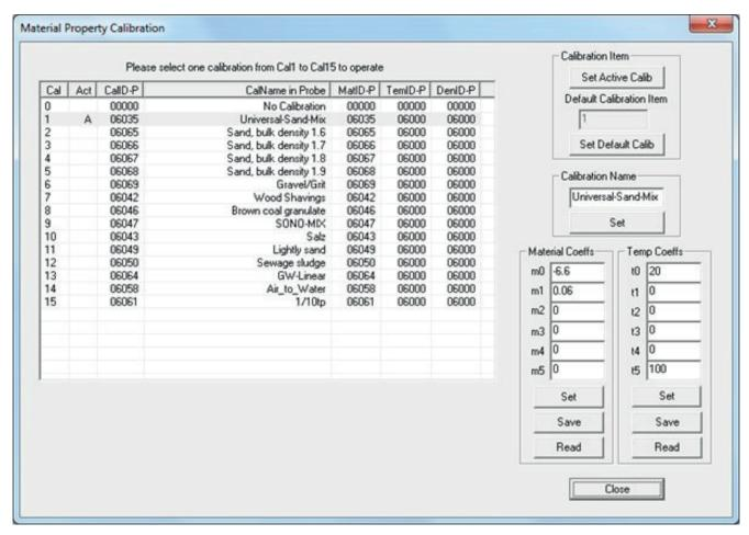
The desired and possibly altered calibration curve (Cal1. .15) which is activated after switching on the probes power supply can be adjusted with the button **"Set Default Calib".**
