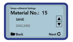
Finally, you can store the calibration into the choosen calibration storage inside the probe. Choose "SAVE" and confirm by pressing the button "Measurement" **C**.
