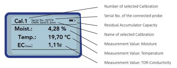
In order to initiate a measurement, shortly press the button "Measurement" C. The measurement will commence and a turning C -symbol will appear instead of the accumulator-symbol in the upper right hand corner. During this period, no other actions can be performed. The measurement requires approximately 4 to 5 seconds.
