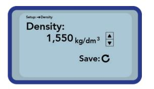
Adjust the density of your material by actuating the buttons "Up" 🛆 and "Down" 🔽. Confirm your setting by pressing the button "Measurement" C. You will get back to the measurement screen. Leave the setting without changing the density by pressing the button "Settings" 🗁
