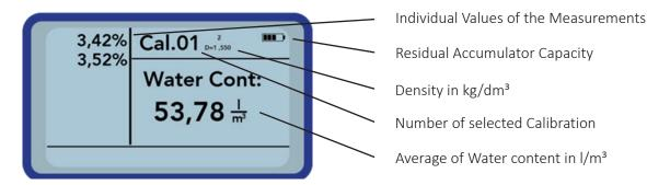
In order to delete the measurement series, actuate the button "Down"  $\square$ .
