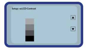
Change the contrast by actuating the button "Up" ▲, respectively "Down" ☑. Set the contrast that you can realize the whole grayscale on the diagram. Activate and store your settings by actuating the button "Measurement" ☑. After activation, the symbol 📺 will appear in the upper right hand corner of the display.
