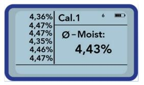
Within the operating mode "Average Value", the HD2 will deliver a representative measurement result for the volume of the material.
