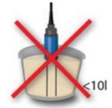
• The bucket should be as far as possible cylindrical, to prevent compaction of the material
