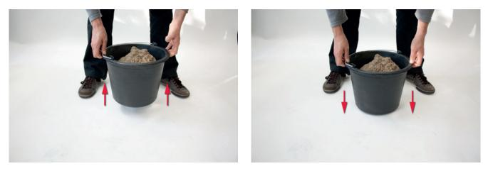
3. Sand: Insert the probe rods into the sand completely, until the gray probe body reaches the surface of the sand and press until you feel counter pressure of the sand (neither jiggle nor rotate the probe while inserting)
