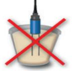
• The filling depth of the bucket must exceed the rod length by minimum 5cm
