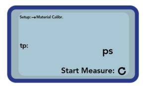
To start the measurement of the material press the button "Measurement" **G**. To improve the accuracy, four measurements will be taken.
