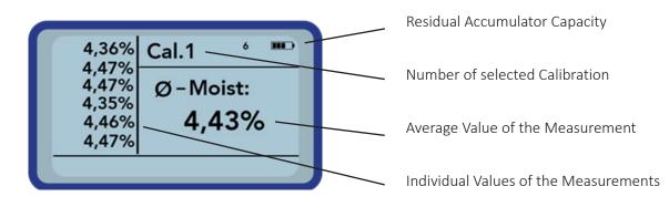
In order to initiate a measurement, shortly press the button "Measurement" C. The measurement will commence and a turning C -symbol will appear instead of the accumulator-symbol in the upper right-hand corner. During this period, no other actions can be performed. The measurement requires approximately 4 to 5 seconds.
