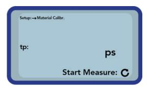
To start the measurement of the material press the button "Measurement" **G**. To improve the accuracy, four measurments will be taken. The individual values are averaged. The duration of a measurement takes around 20 seconds. After each measurement the signal runtime will be displayed for a short period.
