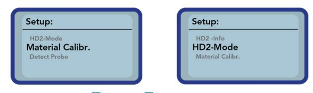
By actuating the buttons "Up"  $\bigtriangleup$  and "Down"  $\bigtriangledown$ , the entry intended for processing can be marked and subsequently be selected with the button "Measurement"  $\bigcirc$ . You can exit the current menu item and also the menu "Settings", with the button "Settings"  $\succeq$ .
