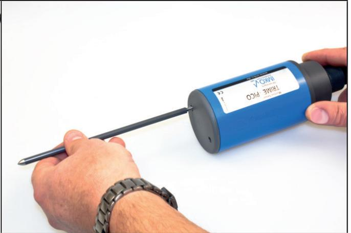
A hand is shown screwing one of the black probe rods into the front of the blue probe body.     |
