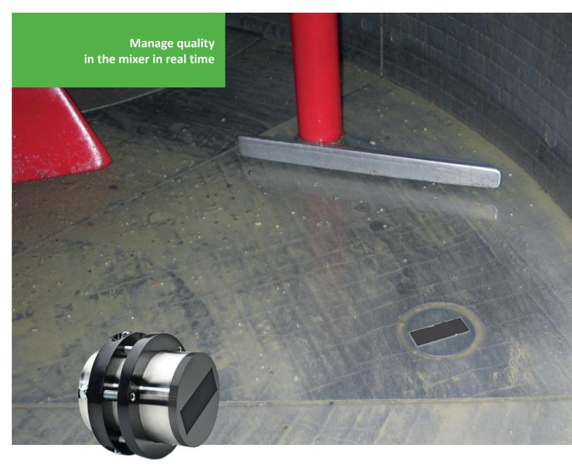
Based on the innovative TRIME radar technology, the determination of water contents during the mixing of concrete is possible: Without value drift over lifespan and wear of the probes.
