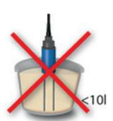
• The bucket should be as far as possible cylindrical, to prevent compaction of the material
