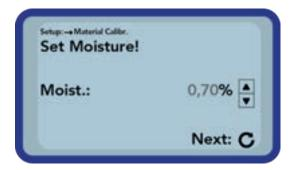
Next set the moisture of the material by pressing the buttons "Up"  $\triangle$  and "Down"  $\checkmark$ . Apply your setting by actuating the button "Measurement"  $\checkmark$ .
