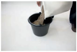
2. Compact the sand sample by lifting the bucket 5cm and letting it fall down vertically onto a solid base and repeat this procedure 5 times (if you still observe compaction after 5-times, repeat this procedure until there is no more compaction to see!)
