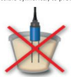
• The filling depth of the bucket must exceed the rod length by minimum 5cm
