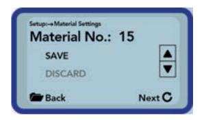
Finally, you can store the calibration into the choosen calibration storage inside the probe. Choose "SAVE" and confirm by pressing the button "Measurement" G.
